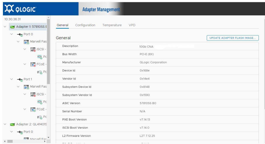
Figure 5-3. Adapter Management of Single-Function 578xx/41000 Series Adapters
